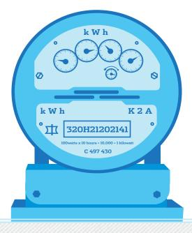
A 100-watt bulb that is turned on for 10 hours uses 1 kWh of electricity (100 watts x 10 hours = 1000 watt-hours divided by 1000 watts/kilowatt = 1 kWh)
