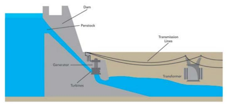
Hydropower is the process of changing the energy of moving water into electrical energy. Graphic courtesy of Bismarck State College National Energy Center of Excellence.
