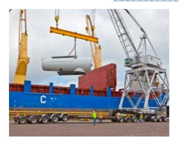
A wind turbine nacelle is loaded off a ship in Duluth Harbor. Photo courtesy of Minnesota Power.
